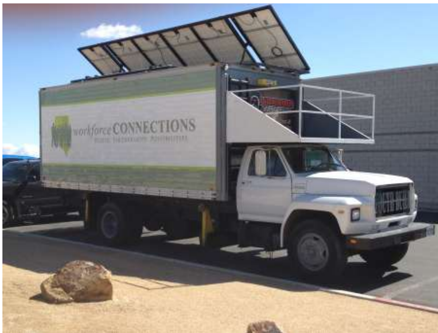
The Green Mobile Classroom is equipped with STEM interactive labs and hands-on activities. The classroom is powered by solar energy (see photo-voltaic panels on the roof).
